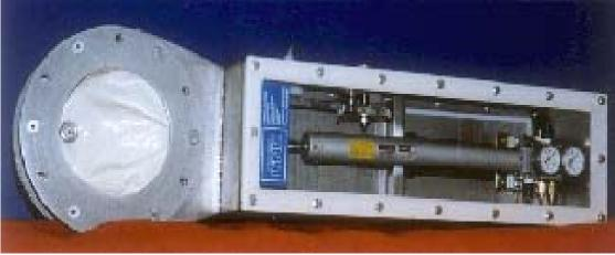
This version of the Membrane Slide Valve is fitted with a sophisticated, infinitely adjustable, positioning cylinder. This enables the valve to open to any position required when given a 3-15 psi pneumatic signal, or a 4-20mA electrical signal.
